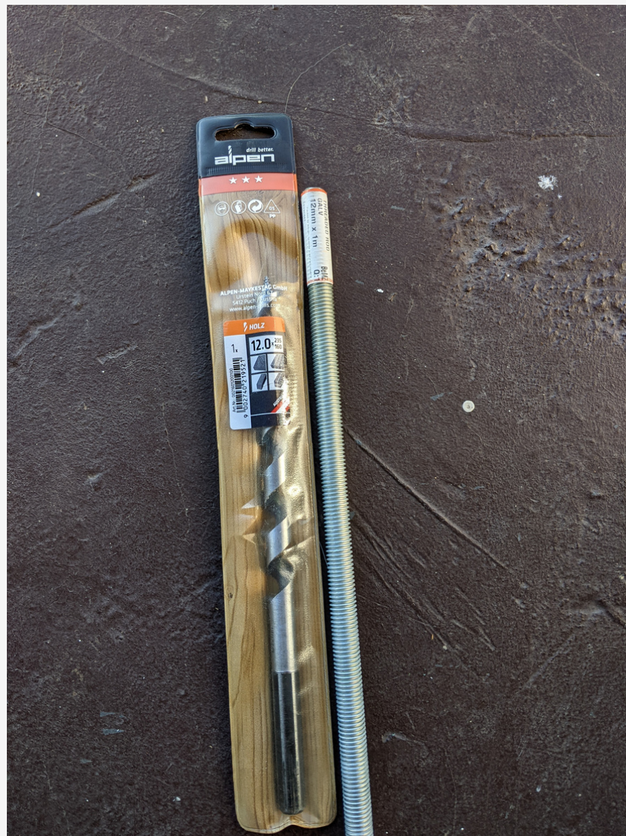
Wood drill bit and portion of threaded rod. Use a drill bit that is the size of your threaded rod.
